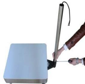
Step 2: After threading the Load Cell wire through the bracket (3), attach the bracket to the upright pole and then lock it with the screw (6).
