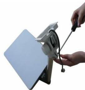
Note: if the load cell connector is too big to thread through the bracket, separate the bracket by removing the knob pole (7), see the following pictures.
