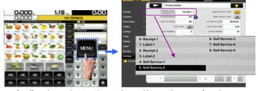
In the case of self-service scales, to change the working mode, press four times consecutively and alternatively between the lower left side and the lower right side of the keypad.
