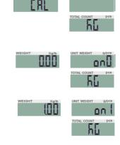
If you need to change the value, do as the following: Press key *G N/SET* to enter the value setting. Press key *√MR* or *TARE/* to move leftwards or rightwards. Press key *M-/HI* or *PRINT/LO* to modify the value (or via numeric keys). Press key
